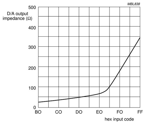
b. Output impedance near positive power rail; T<sub>amb</sub> = +27° C.
