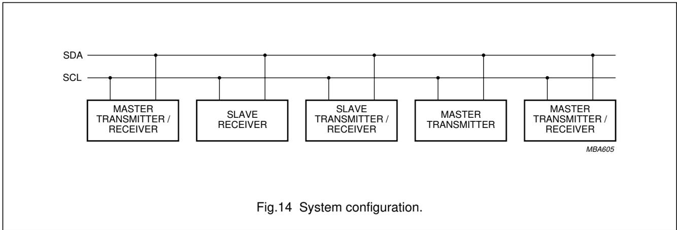
Fig.14 System configuration.
