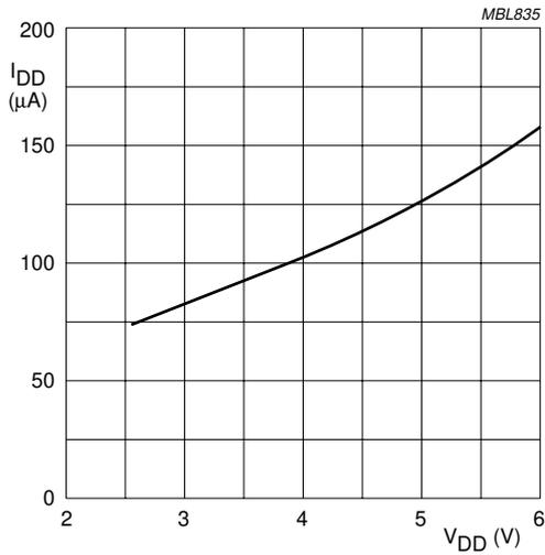
a. Internal oscillator; T<sub>amb</sub> = +27° C.
