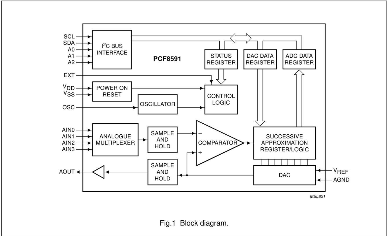
Fig.1 Block diagram.
