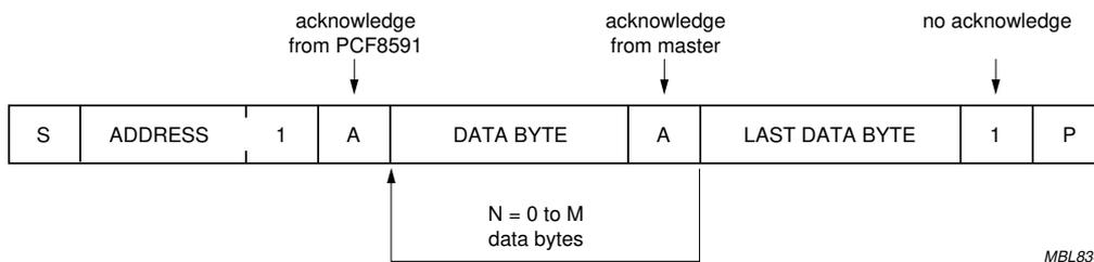
Fig.17 Bus protocol for read mode, A/D conversion.
