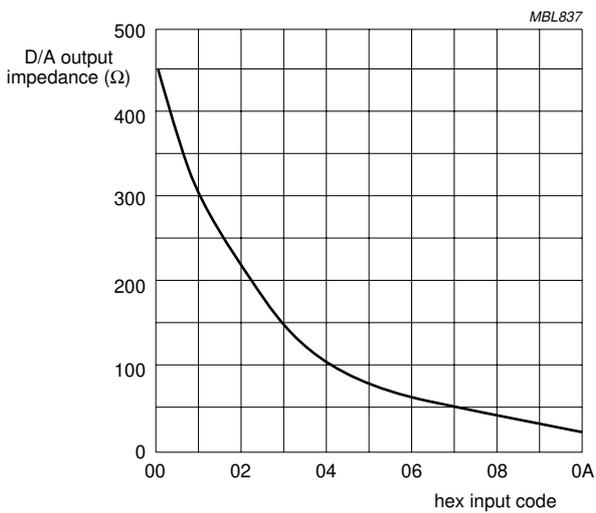
a. Output impedance near negative power rail; T<sub>amb</sub> = +27° C.
