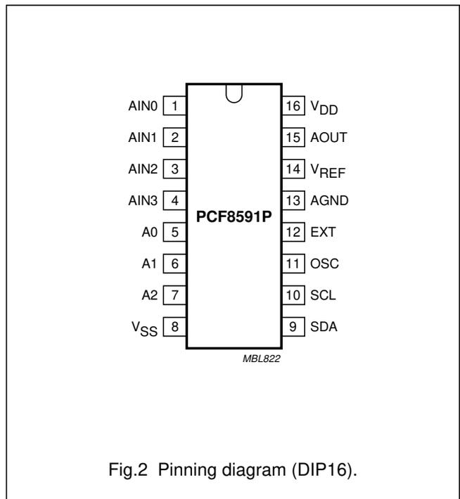
Fig.2 Pinning diagram (DIP16).
