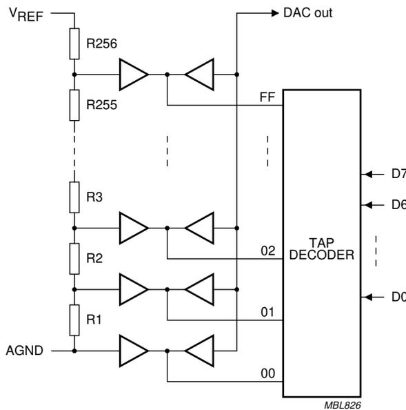
Fig.6 DAC resistor divider chain.
