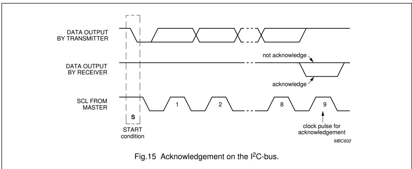
Fig.15 Acknowledgement on the I<sup>2</sup>C-bus.
