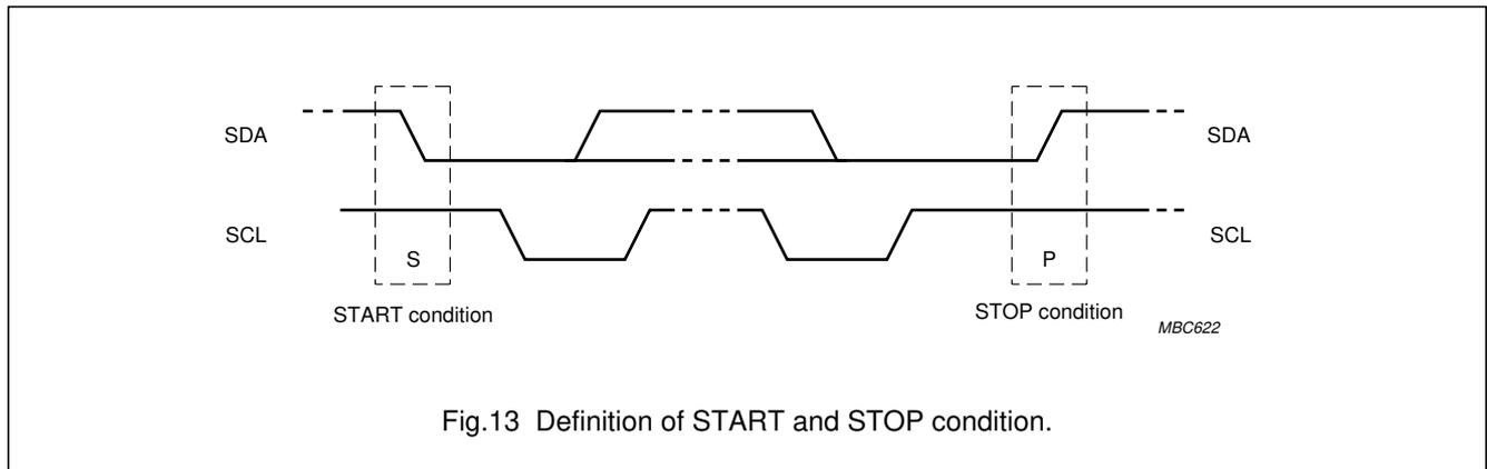
Fig.13 Definition of START and STOP condition.
