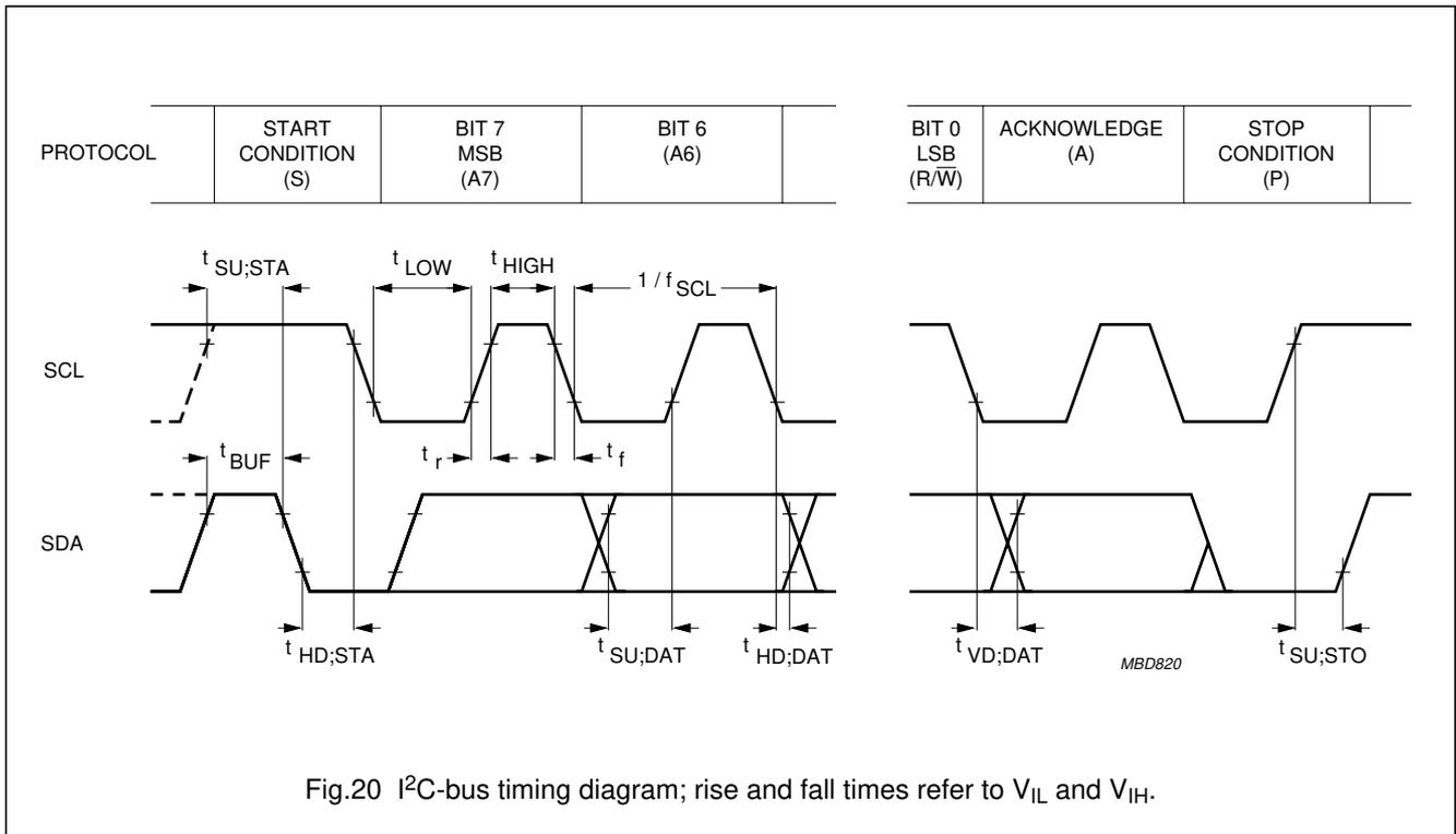
Fig.20 I<sup>2</sup>C-bus timing diagram; rise and fall times refer to  $V_{IL}$  and  $V_{IH}$ .
