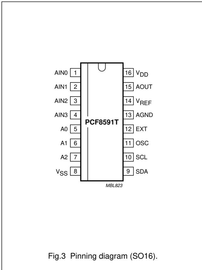
Fig.3 Pinning diagram (SO16).
