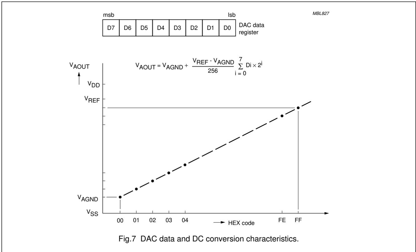
Fig.7 DAC data and DC conversion characteristics.
