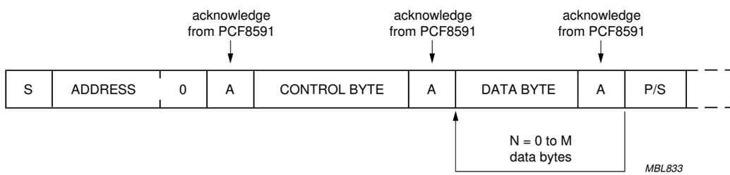
Fig.16 Bus protocol for write mode, D/A conversion.
