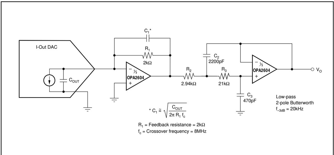
FIGURE 5. DAC I/V Amplifier and Low-Pass Filter.
