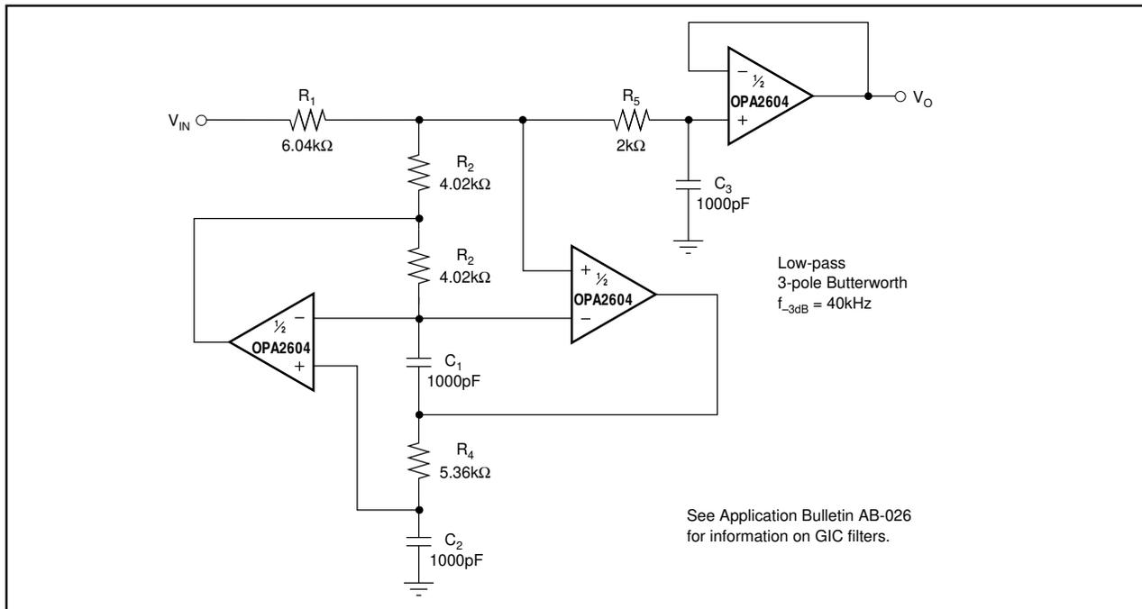
FIGURE 4. Three-Pole Generalized Immittance Converter (GIC) Low-Pass Filter.
