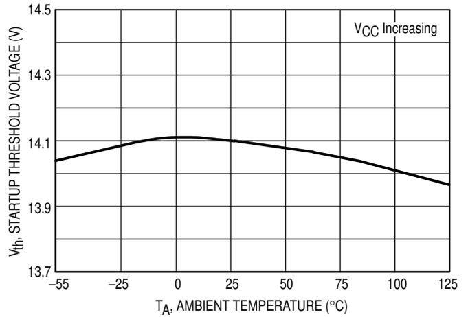
Figure 25. Minimum Operating Voltage After Turn-On versus Temperature
