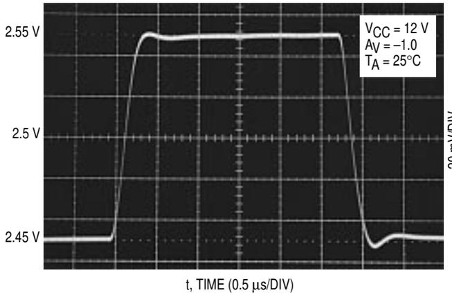
Figure 6. Error Amp Large Signal Transient Response
