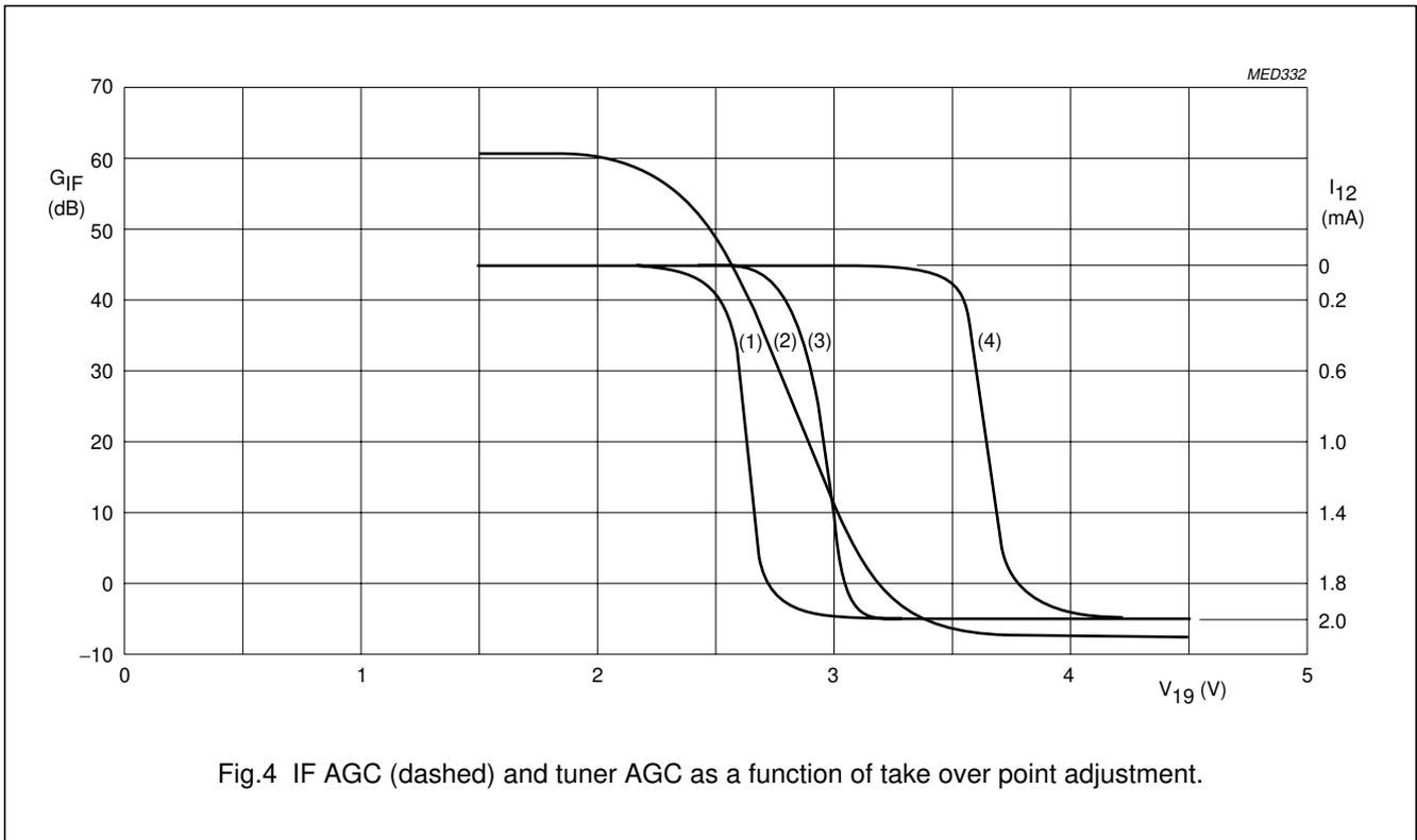
Fig.4 IF AGC (dashed) and tuner AGC as a function of take over point adjustment.
