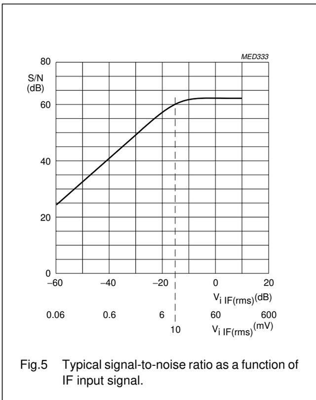
Fig.5 Typical signal-to-noise ratio as a function of IF input signal.
