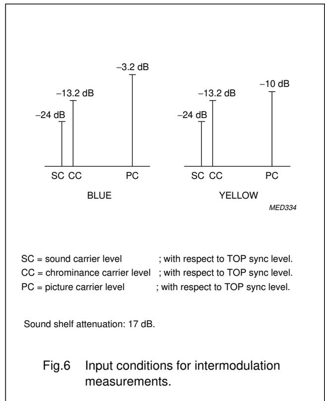
SC = sound carrier level ; with respect to TOP sync level.
