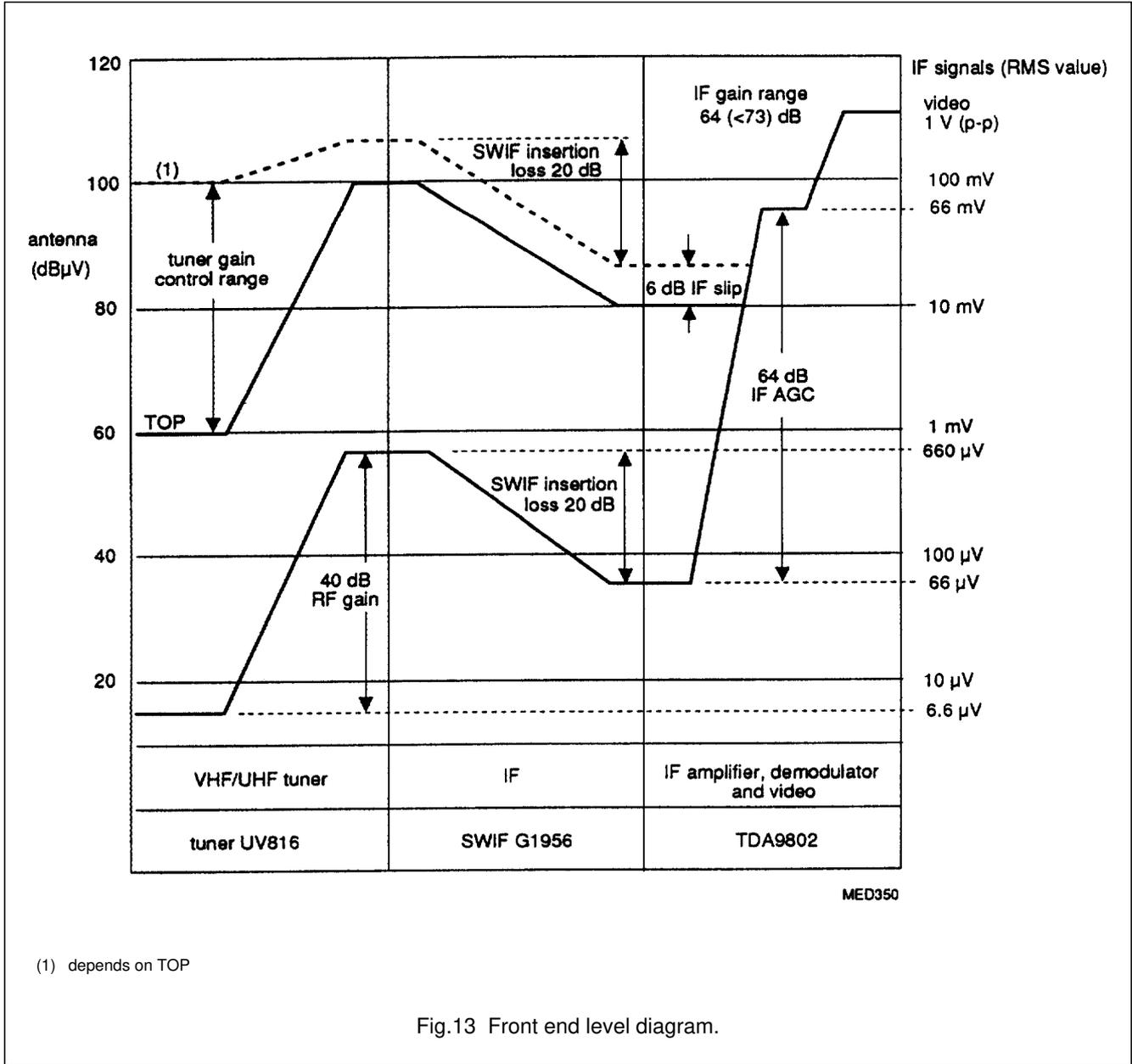
Fig.13 Front end level diagram.
