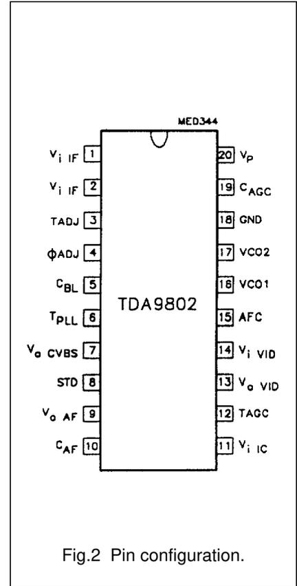
Fig.2 Pin configuration.
