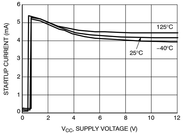
Figure 18. Startup Current vs. V<sub>CC</sub> Voltage
