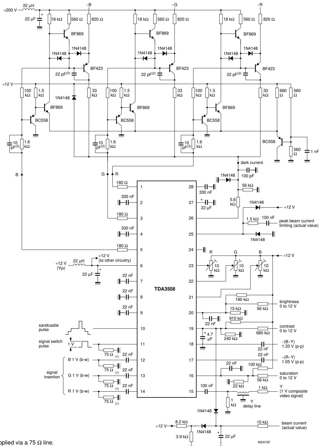
Fig.4 Typical application circuit diagram using TDA3508; colour difference inputs are negative.
