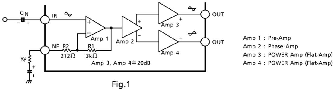
This IC has the amplifier construction as shown in Fig.1. The pre-amp. Amp 1 is provided to the primary stage, and the input voltage is amplified by the flat amps, amp 3 and amp 4 of each channel through the phase amp. Amp 2.
