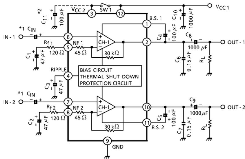
(\*1): This IC can be used without coupling capacitor ( $C_{IN}$ ). If volume slide noise occurred by input offset voltage is undesirable, it needs to use the capacitor ( $C_{IN}$ ).
