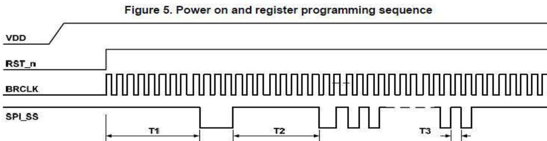
1. After VDD power is ready, make sure to have valid reset on pin RST\_n, which is active-low.
