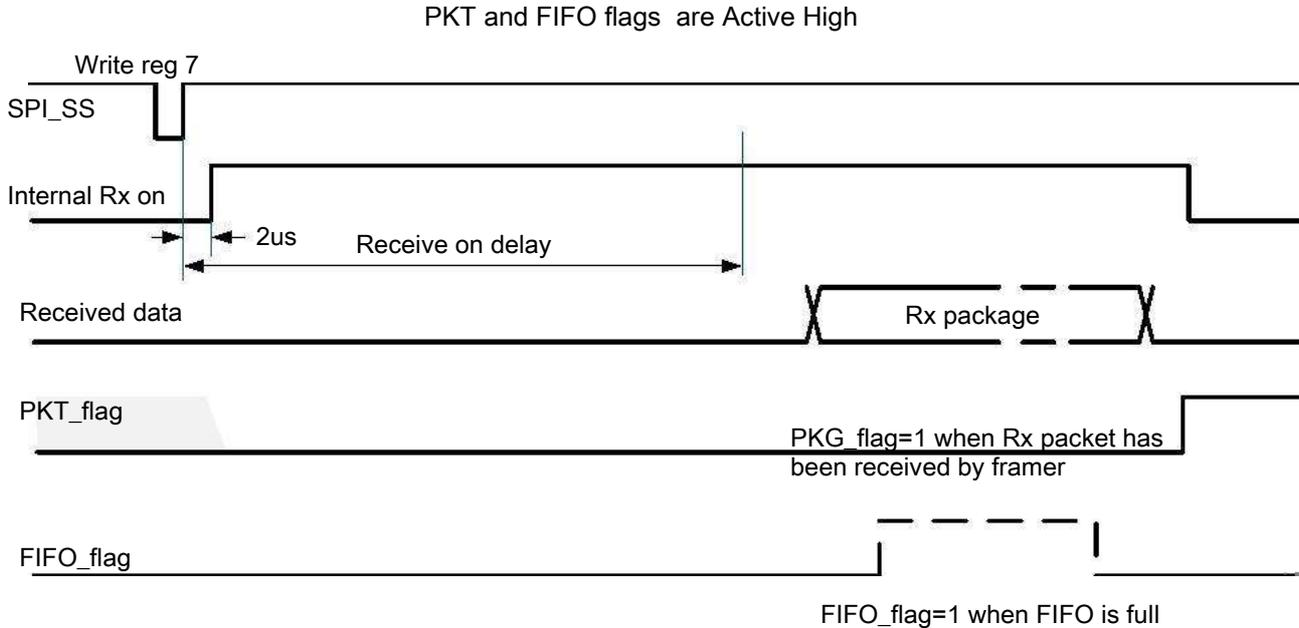
Figure 10. Example Rx packet flowchart
