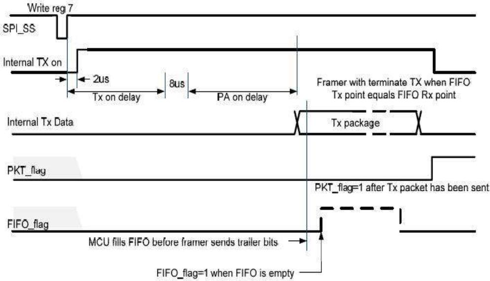
Note: When Register 41[13] = 0 (MCU/application handles packet length), never let FIFO underflow or over flow. FIFO full/empty thresholds can be controlled via Register 40 FIFO\_EMPTY\_THRESHOLD and FIFO\_FULL\_THRESHOLD settings. The best value will depend on SPI speed, and speed at which MCU/application can stream the data into FIFO.
