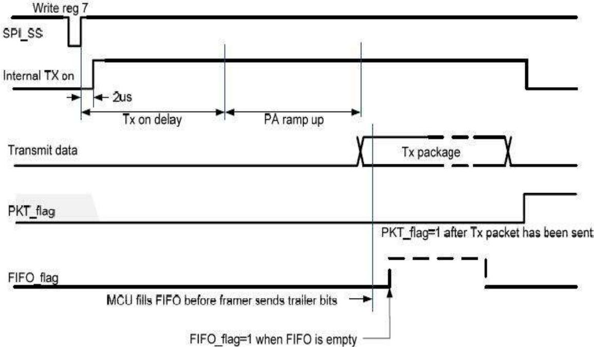
Figure 8. Example Tx packet flowchart
