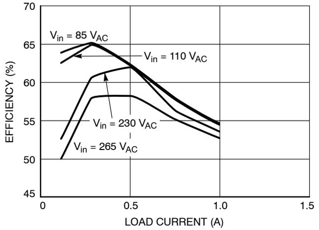
Figure 37. Charger Efficiency
