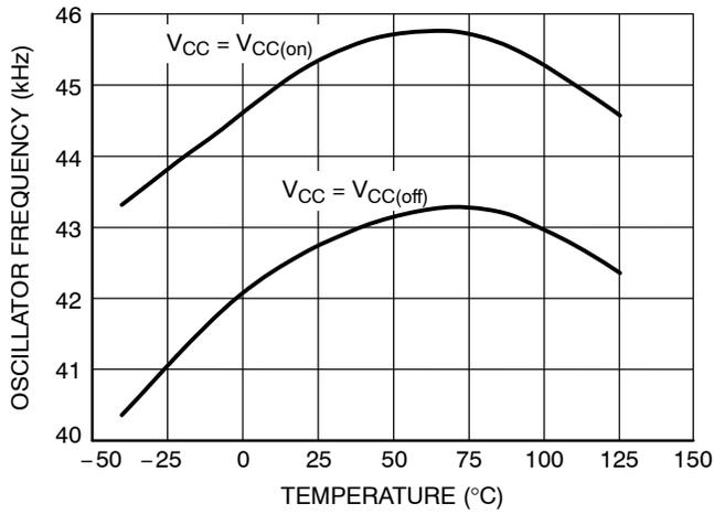
**Figure 5. Oscillator Frequency (44 kHz Version) versus Temperature**
