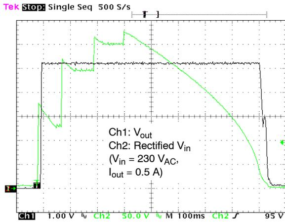
Figure 38. Converter On/Off Line Transient Response
