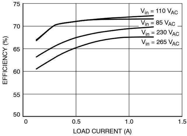
Figure 36. Converter Efficiency
