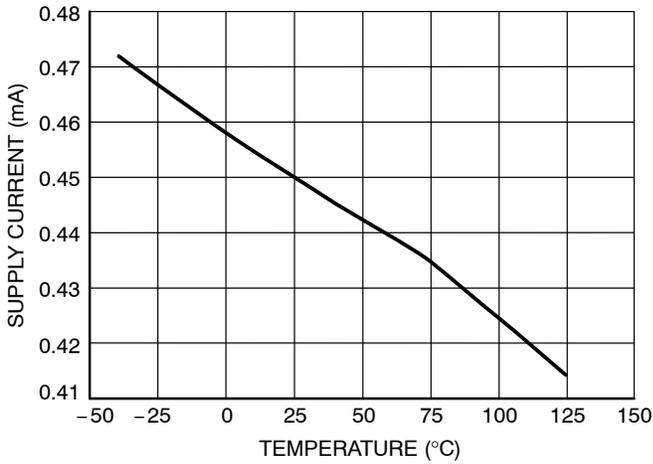
**Figure 25. Supply Current When Switching Disable versus Temperature**
