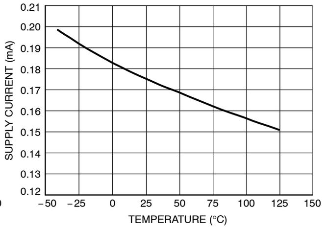
**Figure 26. Supply Current in Fault Condition versus Temperature**
