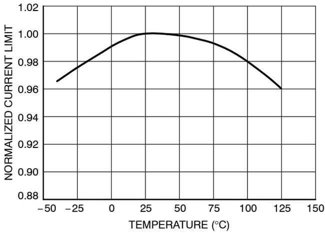
Figure 17. Normalized Peak Current Limit versus Temperature
