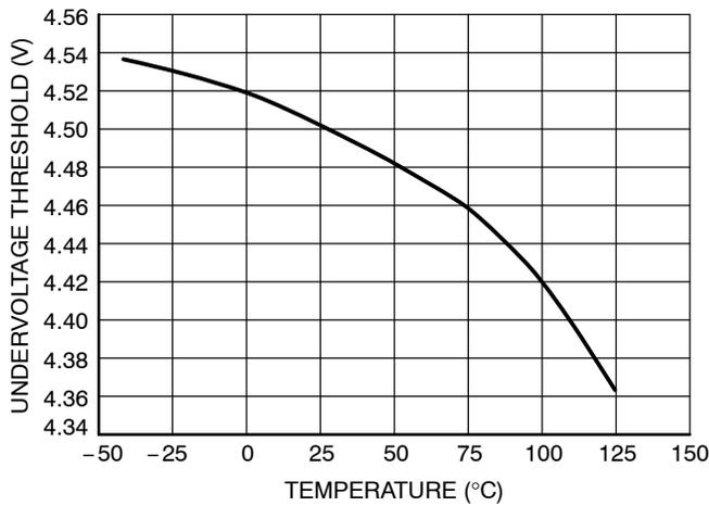
Figure 19. Undervoltage Lockout Threshold versus Temperature
