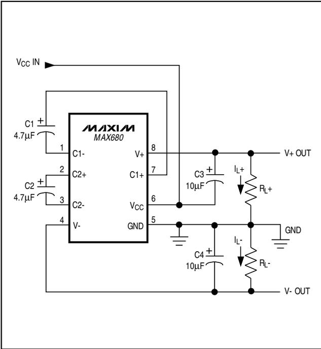
Figure 1. Test Circuit
