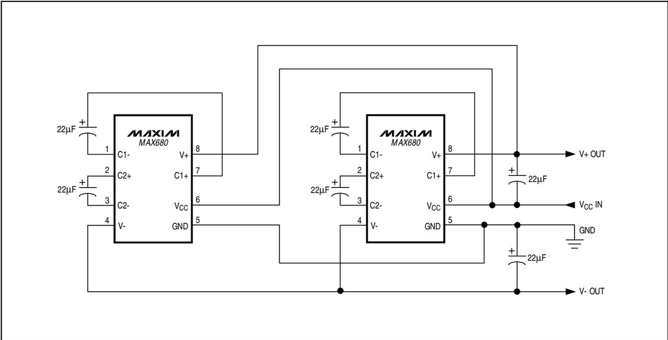
Figure 4. Paralleling MAX680s For Lower Source Resistance
