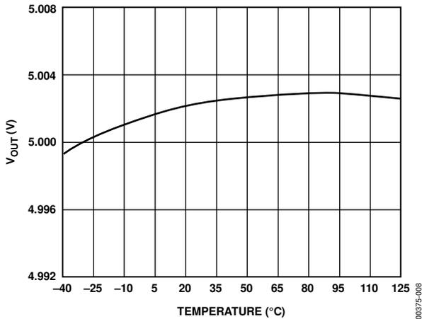
Figure 8. REF02 Typical Output Voltage vs. Temperature
