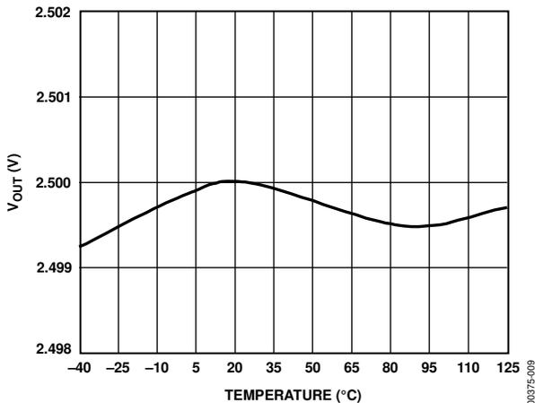
Figure 9. REF03 Typical Output Voltage vs. Temperature
