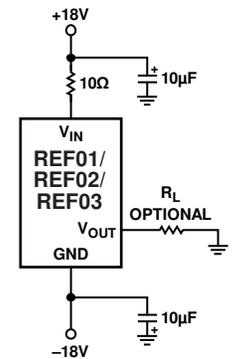
Figure 37. Burn-In Circuit
