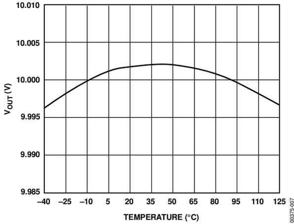
Figure 7. REF01 Typical Output Voltage vs. Temperature
