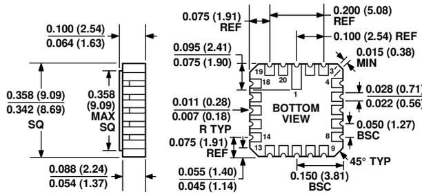
CONTROLLING DIMENSIONS ARE IN INCHES; MILLIMETER DIMENSIONS (IN PARENTHESES) ARE ROUNDED-OFF INCH EQUIVALENTS FOR REFERENCE ONLY AND ARE NOT APPROPRIATE FOR USE IN DESIGN.
