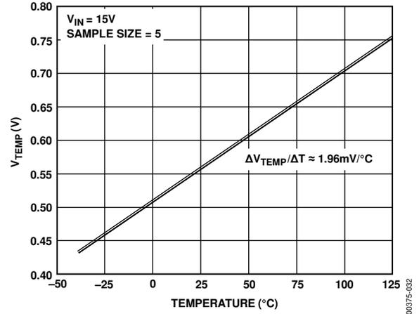
Figure 32. Output Voltage at TEMP Pin vs. Temperature
