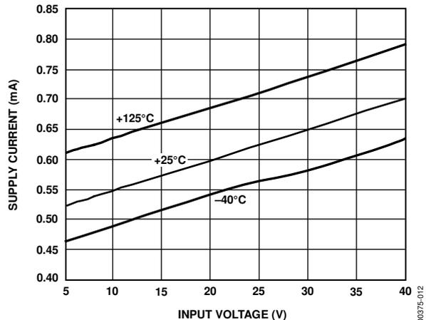
Figure 12. REF03 Supply Current vs. Input Voltage
