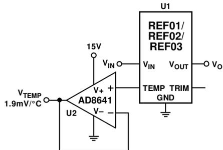
Figure 36. Temperature Monitoring
