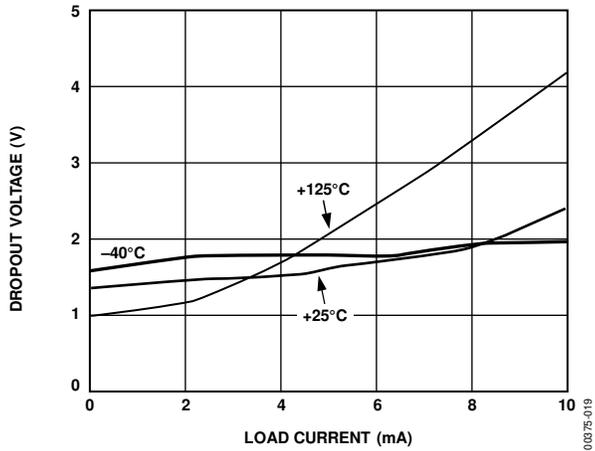
Figure 19. REF01 Dropout Voltage vs. Load Current
