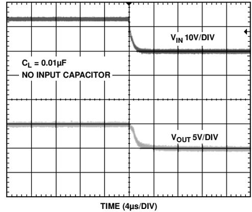
Figure 30. REF02 Turn-Off Response (No Input Capacitor)
