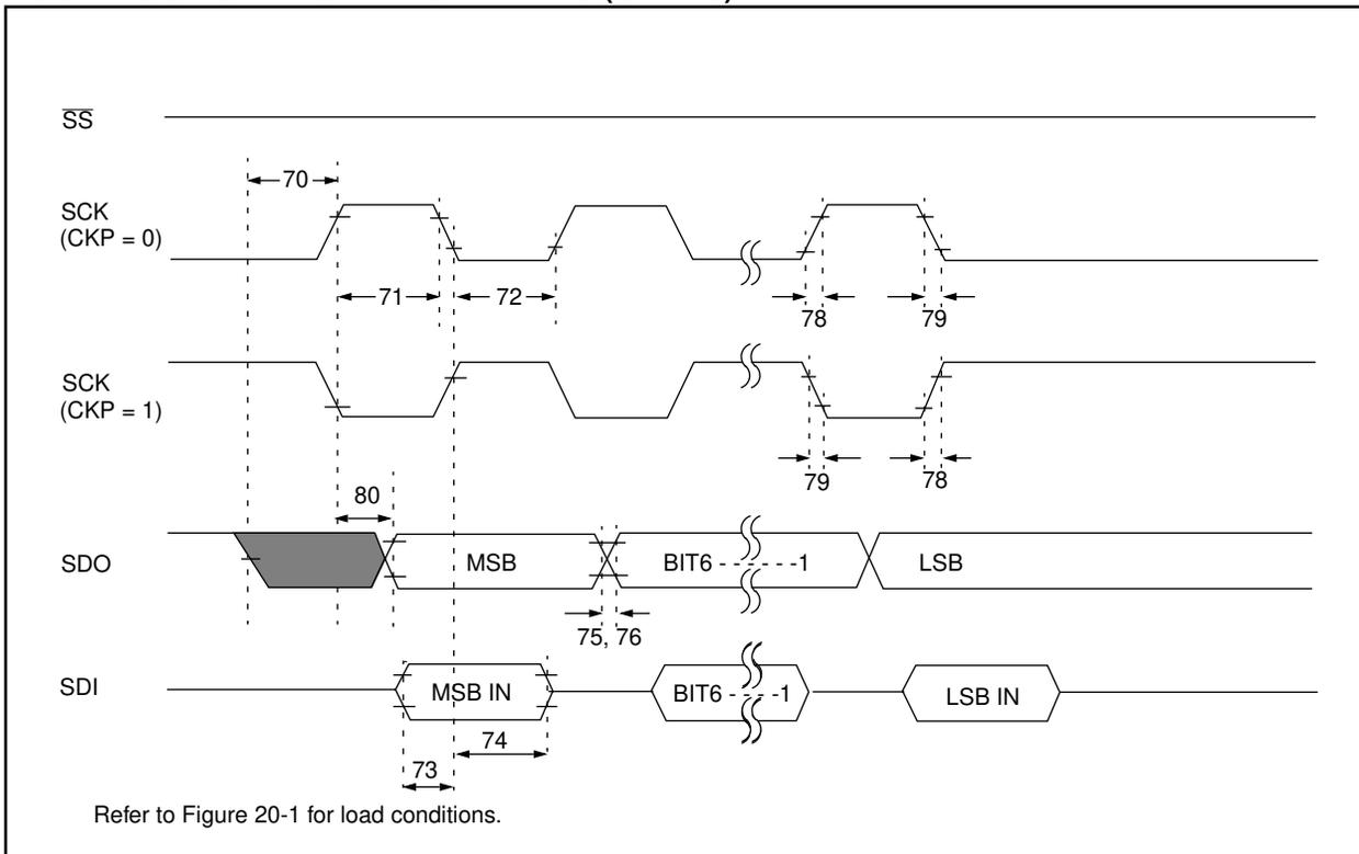
FIGURE 20-10: SPI MASTER MODE TIMING (CKE = 1)
