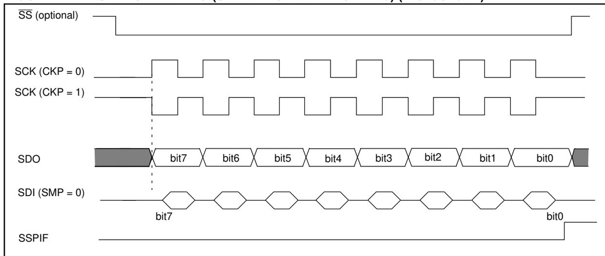
**FIGURE 11-13: SPI MODE TIMING (SLAVE MODE WITH CKE = 1) (PIC16C76/77)**
