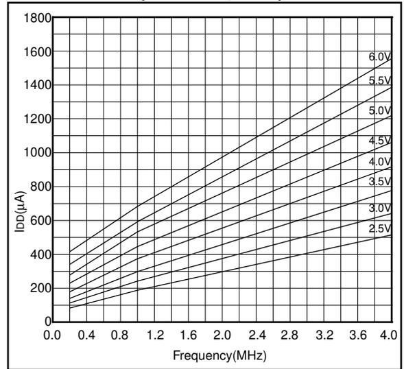
**FIGURE 21-26: MAXIMUM  $I_{DD}$  vs. FREQUENCY (LP MODE, 85°C TO -40°C)**
