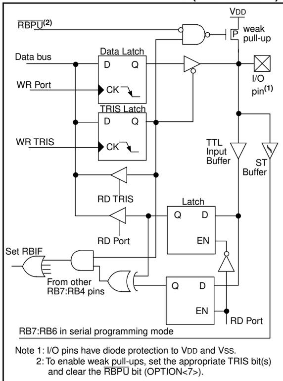
**FIGURE 5-5: BLOCK DIAGRAM OF RB7:RB4 PINS (PIC16C72/73A/74A/76/77)**
