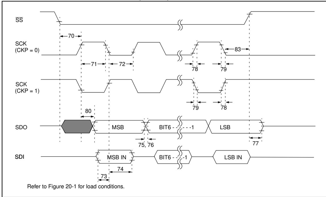
**FIGURE 20-12: SPI SLAVE MODE TIMING (CKE = 1)**
