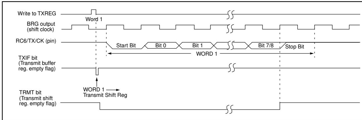
**FIGURE 12-9: ASYNCHRONOUS MASTER TRANSMISSION (BACK TO BACK)**
