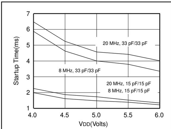
**FIGURE 21-24: TYPICAL XTAL STARTUP TIME vs. VDD (XT MODE, 25°C)**
