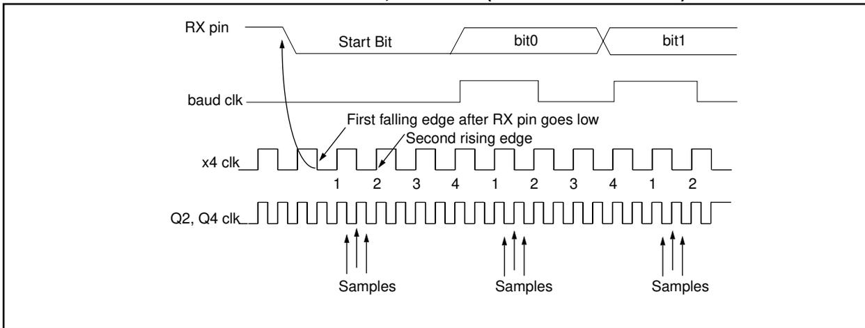
**FIGURE 12-5: RX PIN SAMPLING SCHEME, BRGH = 1 (PIC16C73/73A/74/74A)**
