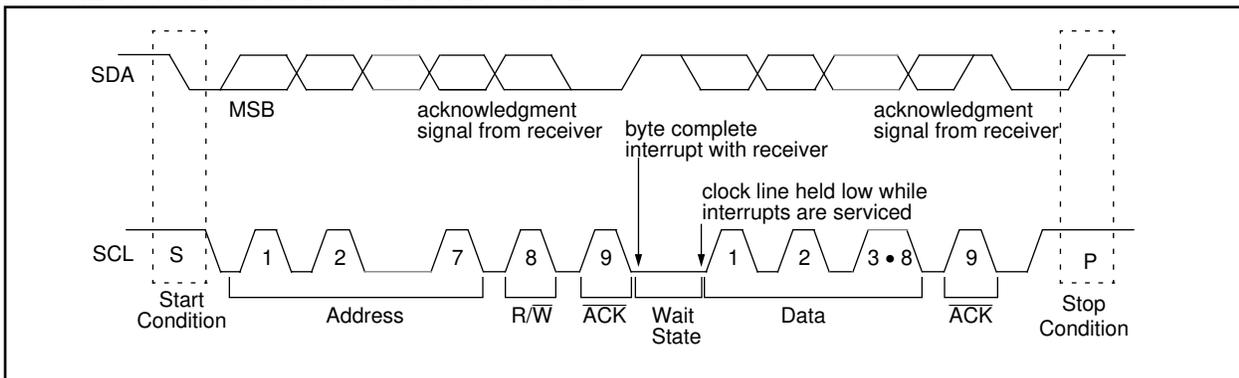
Figure 11-19 and Figure 11-20 show Master-transmitter and Master-receiver data transfer sequences.
