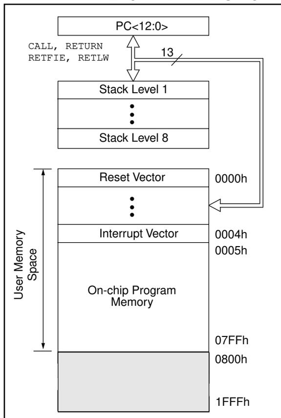
**FIGURE 4-2: PIC16C73/73A/74/74A PROGRAM MEMORY MAP AND STACK**
