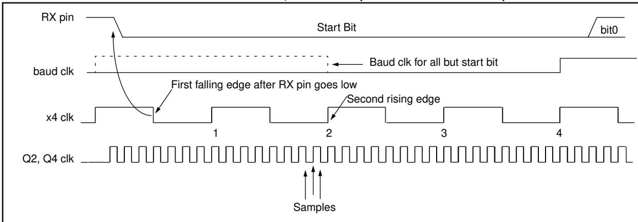
**FIGURE 12-6: RX PIN SAMPLING SCHEME, BRGH = 0 OR BRGH = 1 (PIC16C76/77)**
