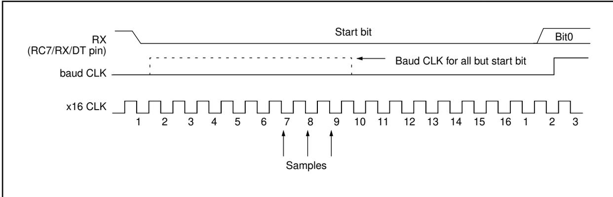
**FIGURE 12-4: RX PIN SAMPLING SCHEME, BRGH = 1 (PIC16C73/73A/74/74A)**
