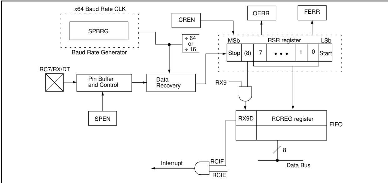
**FIGURE 12-11: ASYNCHRONOUS RECEPTION**
