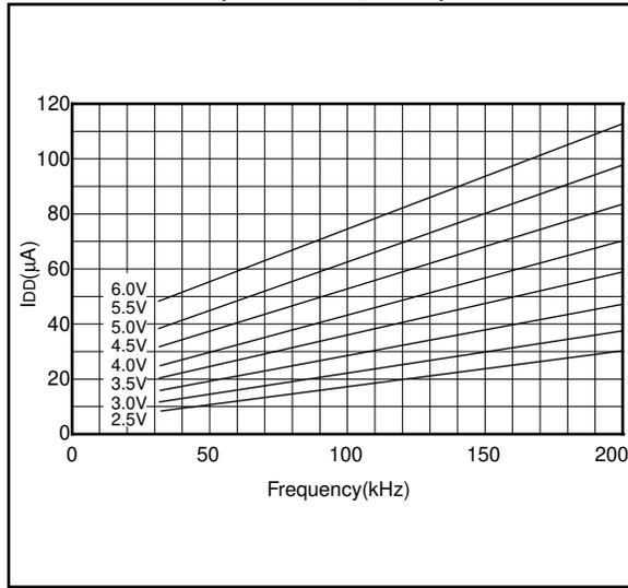
**FIGURE 21-27: TYPICAL  $I_{DD}$  vs. FREQUENCY (XT MODE, 25°C)**
