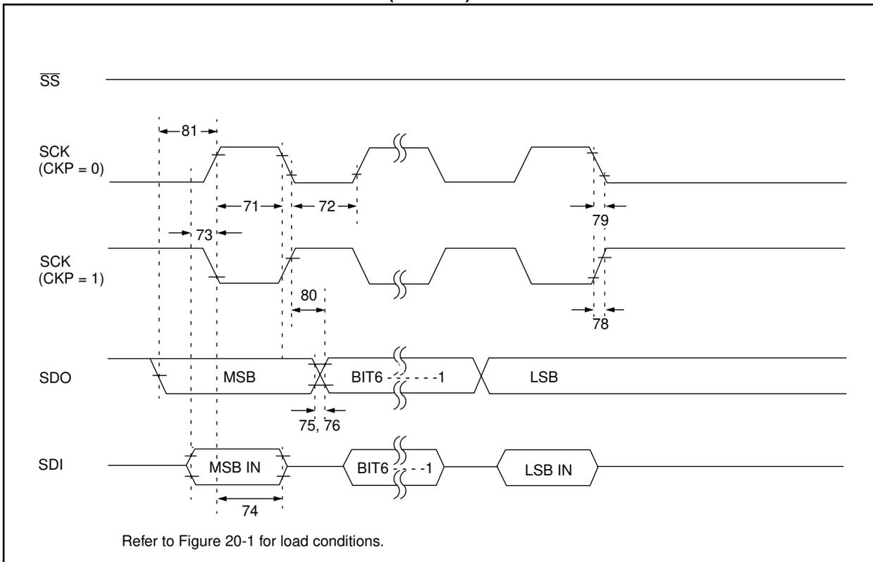
**FIGURE 20-11: SPI SLAVE MODE TIMING (CKE = 0)**
