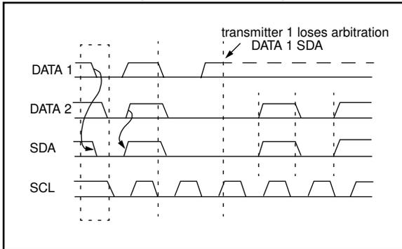
Masters that also incorporate the slave function, and have lost arbitration must immediately switch over to slave-receiver mode. This is because the winning master-transmitter may be addressing it.
