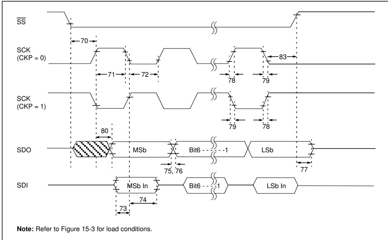
**FIGURE 15-14: SPI SLAVE MODE TIMING (CKE = 1)**
