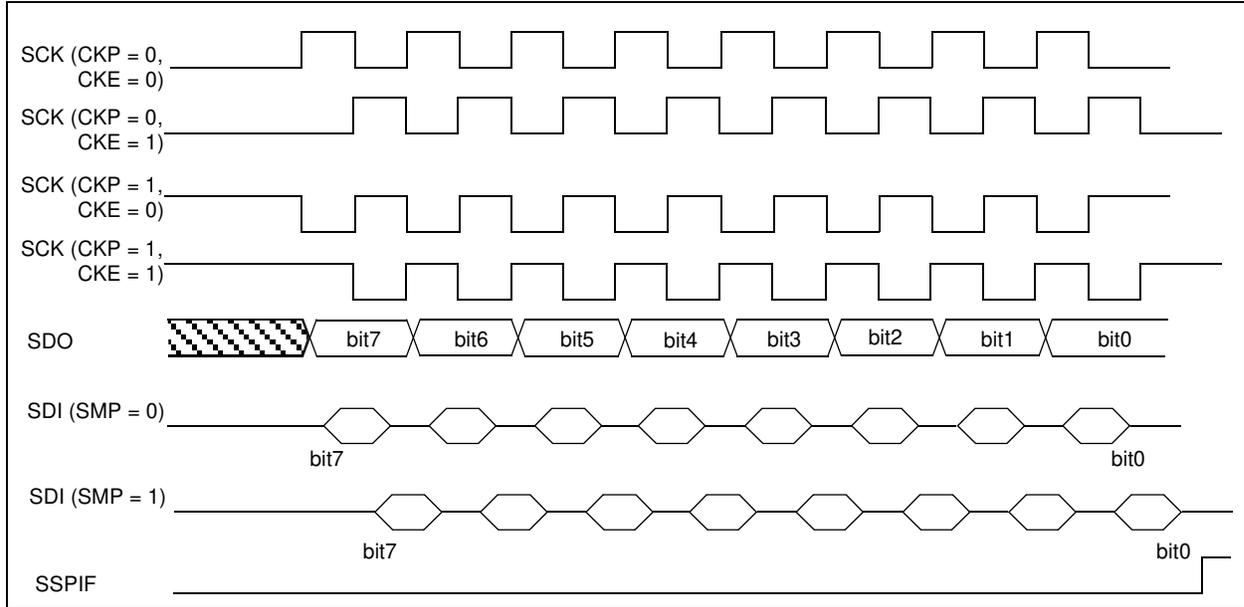
**FIGURE 9-3: SPI MODE TIMING (SLAVE MODE WITH CKE = 0)**
