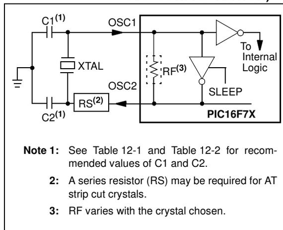
**FIGURE 12-2: EXTERNAL CLOCK INPUT OPERATION (HS OSC CONFIGURATION)**
