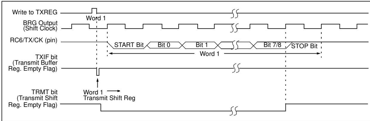
**FIGURE 10-3: ASYNCHRONOUS MASTER TRANSMISSION (BACK TO BACK)**
