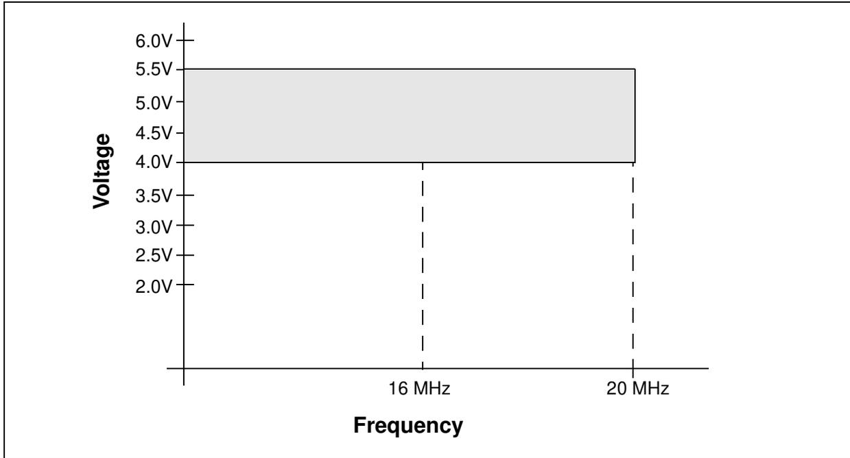
FIGURE 15-2: PIC16LF7X VOLTAGE-FREQUENCY GRAPH
