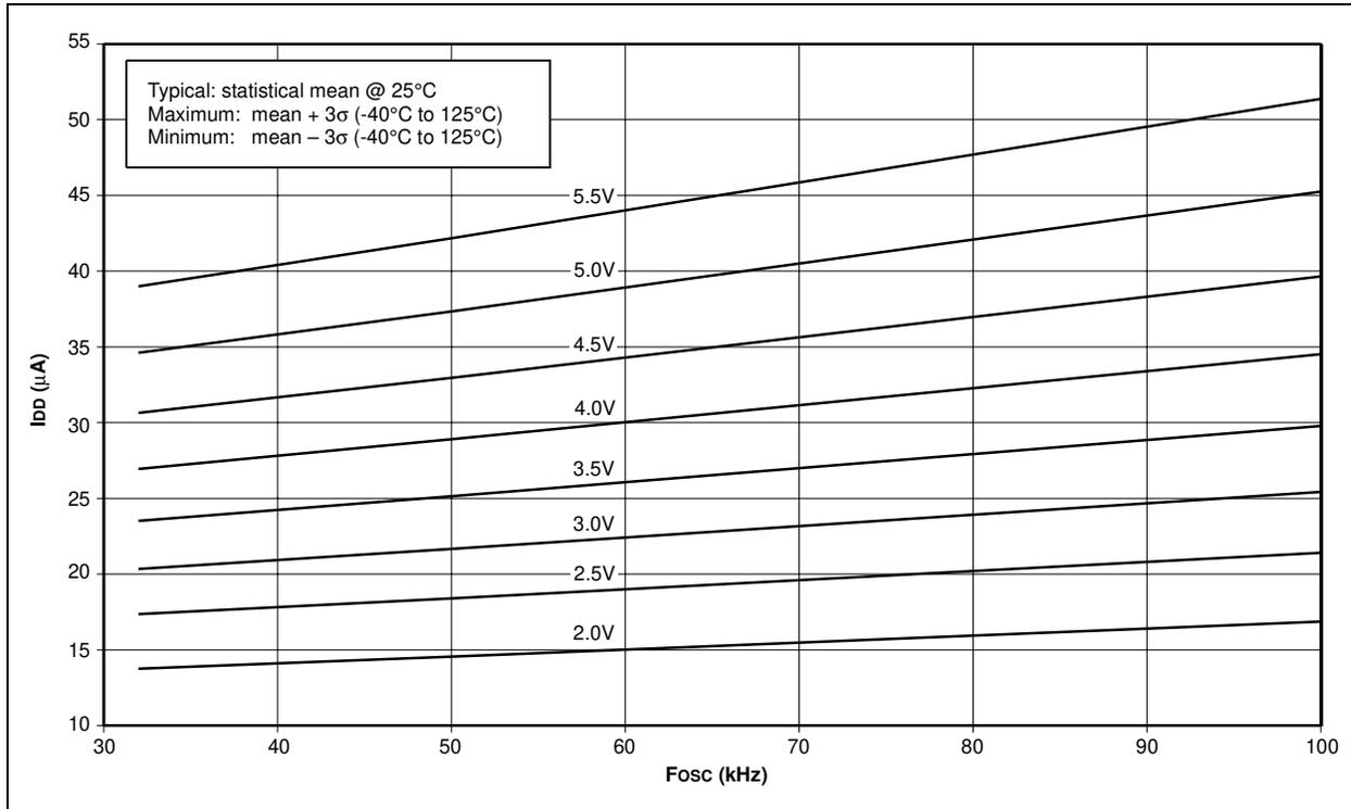
**FIGURE 16-6: MAXIMUM  $I_{DD}$  vs.  $F_{OSC}$  OVER  $V_{DD}$  (LP MODE)**
