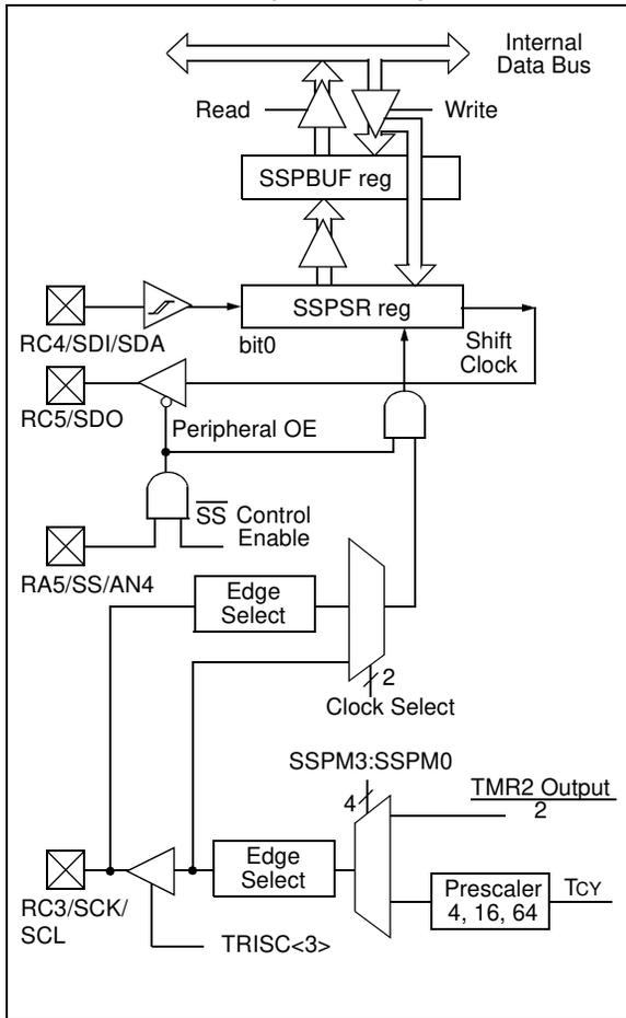
To enable the serial port, SSP enable bit, SSPEN (SSPCON<5>) must be set. To reset or reconfigure SPI mode, clear bit SSPEN, re-initialize the SSPCON register, and then set bit SSPEN. This configures the SDI, SDO, SCK, and SS pins as serial port pins. For the pins to behave as the serial port function, they must have their data direction bits (in the TRISC register) appropriately programmed. That is:
