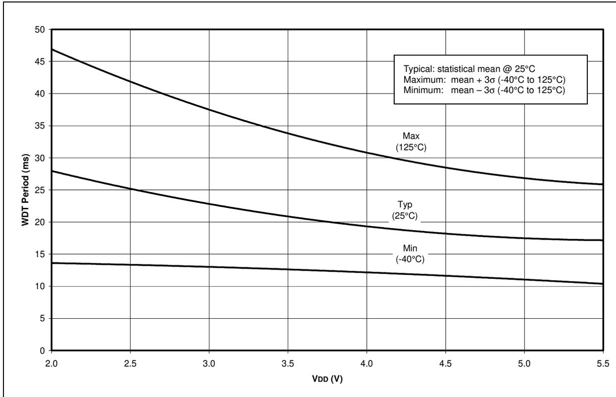
**FIGURE 16-14: AVERAGE WDT PERIOD vs. V<sub>DD</sub> OVER TEMPERATURE (-40°C TO 125°C)**
