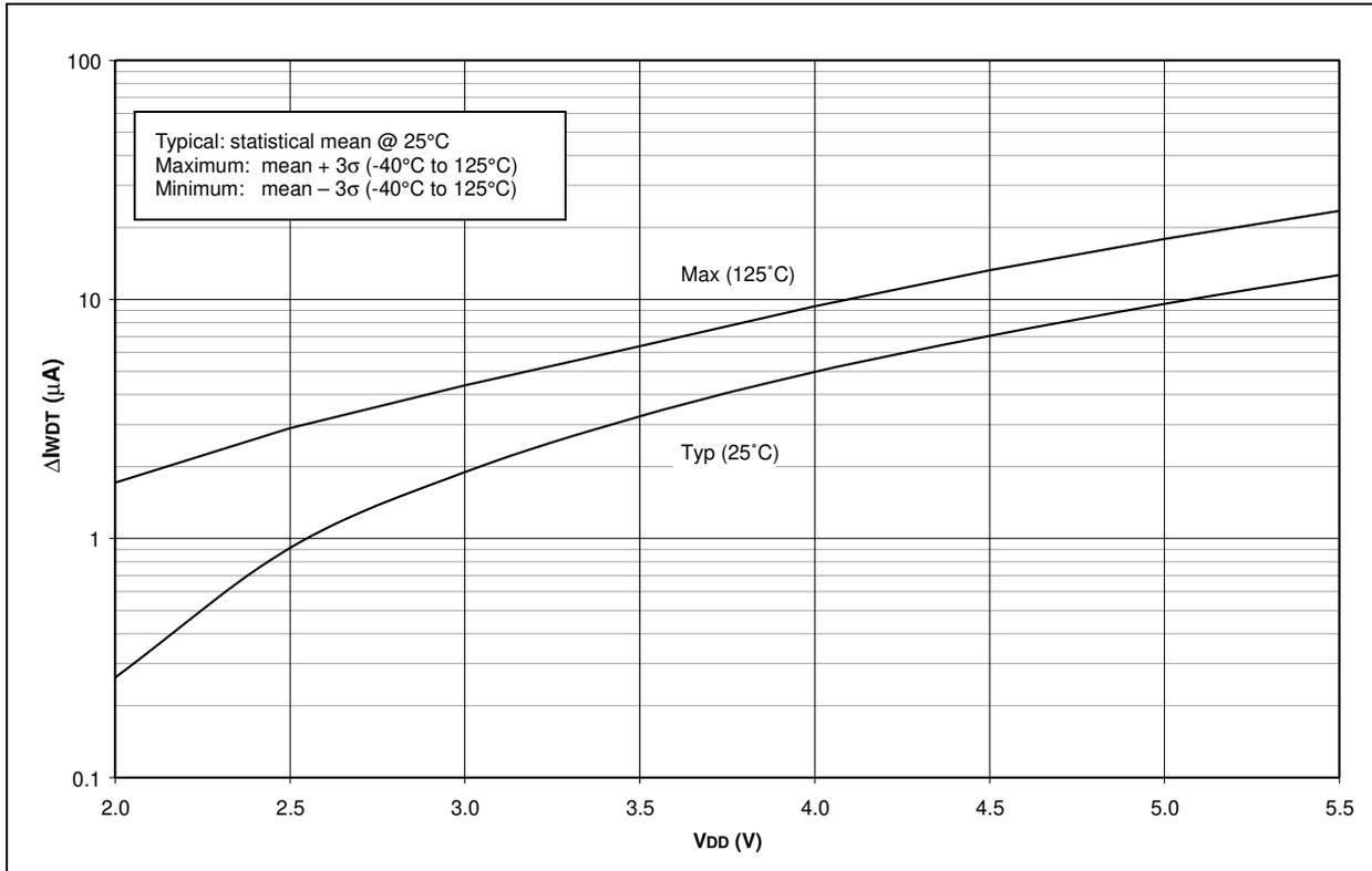
**FIGURE 16-13: TYPICAL, MINIMUM AND MAXIMUM WDT PERIOD vs. V<sub>DD</sub> (-40°C TO 125°C)**
