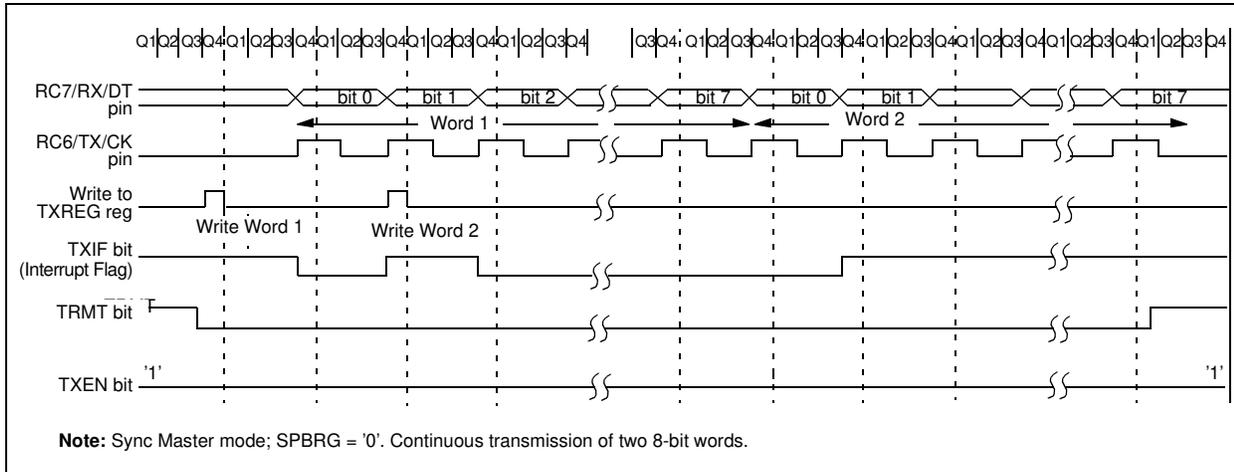
**FIGURE 10-7: SYNCHRONOUS TRANSMISSION (THROUGH TXEN)**
