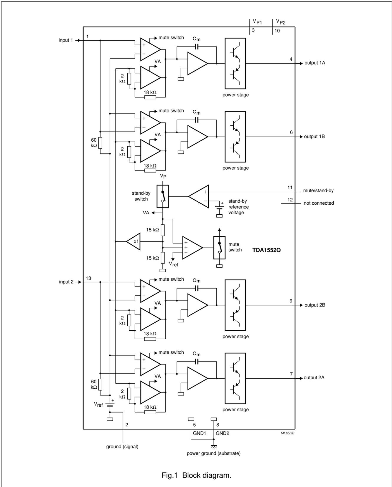
Fig.1 Block diagram.
