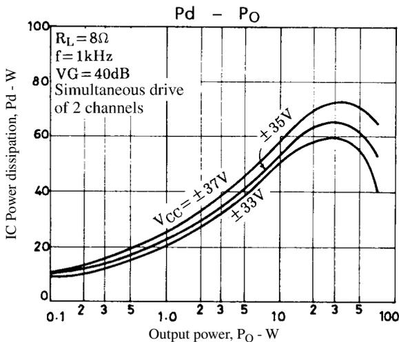
Figure 1. STK4192II Pd - P<sub>O</sub> (R<sub>L</sub> = 8Ω)
