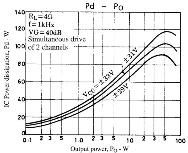
Figure 2. STK4192II Pd - P<sub>O</sub> (R<sub>L</sub> = 4Ω)
