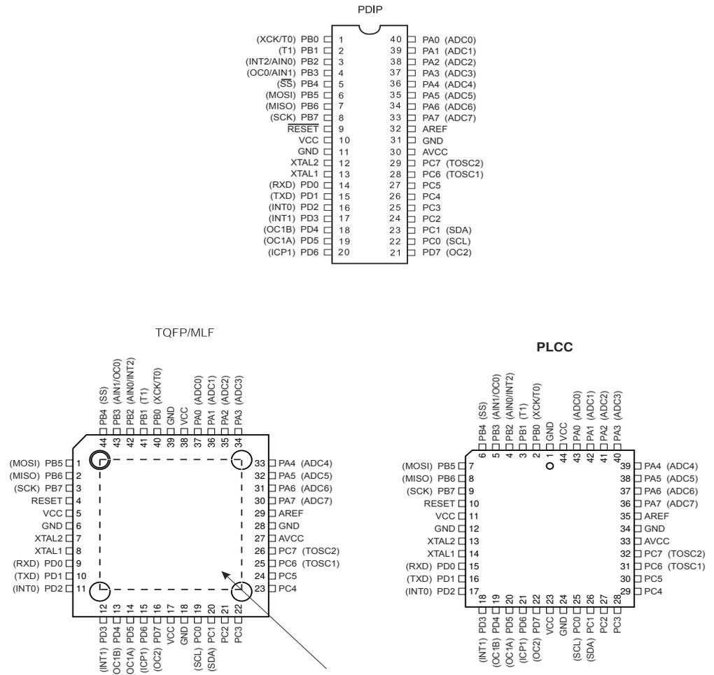
NOTE: MLF Bottom pad should be soldered to ground.
